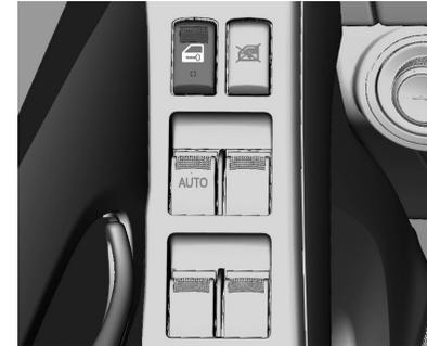
Pulse la parte delantera del interruptor
