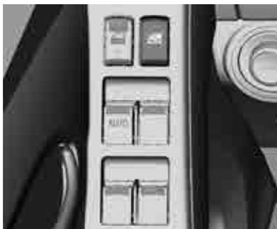
Presione el interruptor
