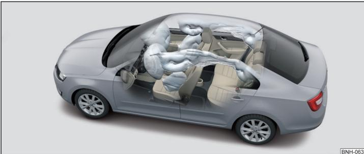
Fig. 21 Airbags rellenos de gas
