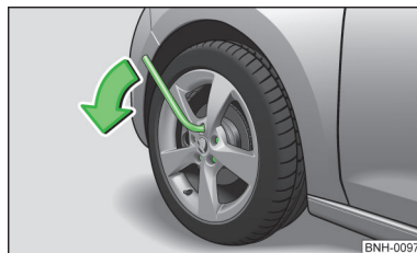
Fig. 90 Loosening the wheel bolts
