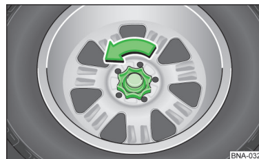
Fig. 87 Removing the wheel
