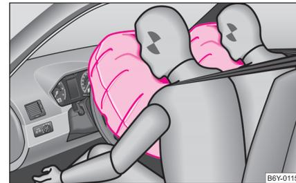
Fig. 127 Airbags rellenos de gas
