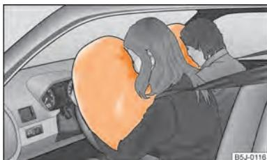
Fig. 98 Airbags rellenos de gas
